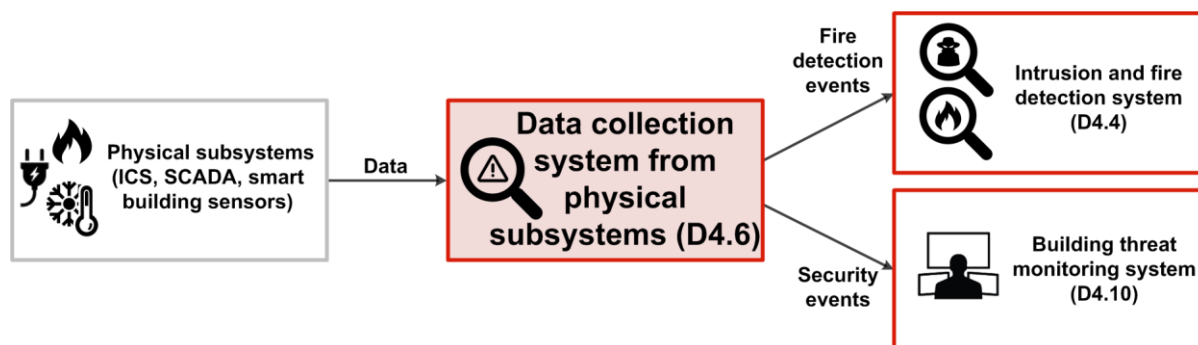
Figure 5 – Interconnections of the data collection system
