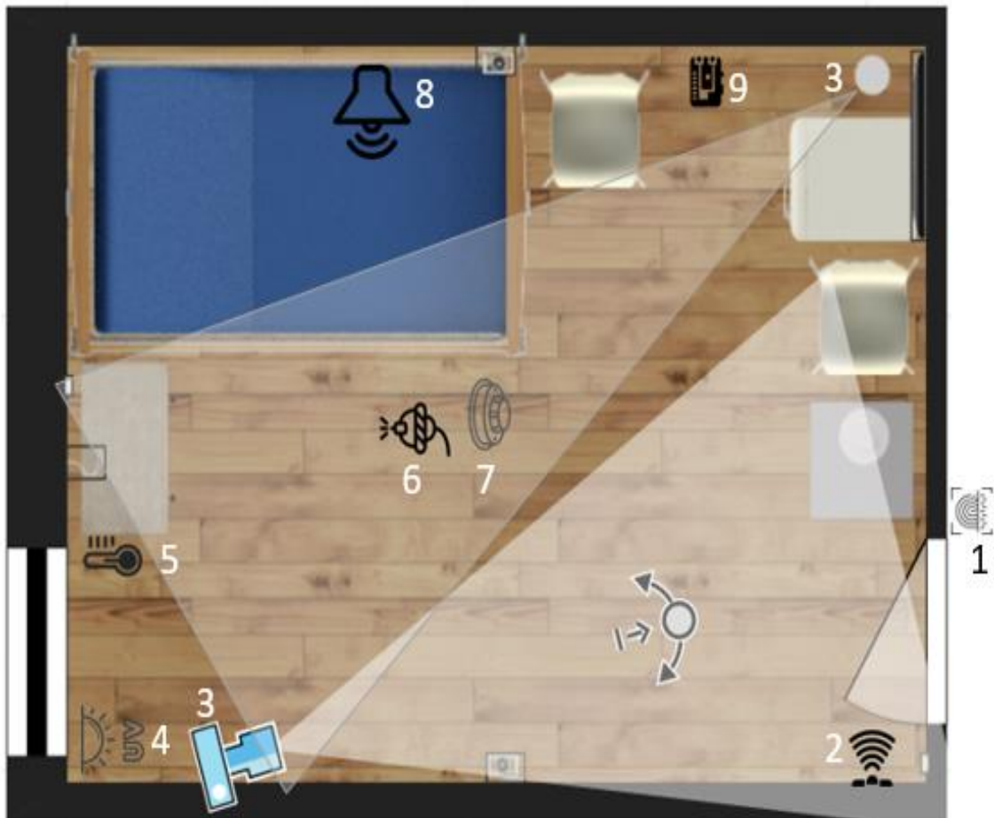
Figure 4 - Schematic representation of sensor placement inside a hospital room
